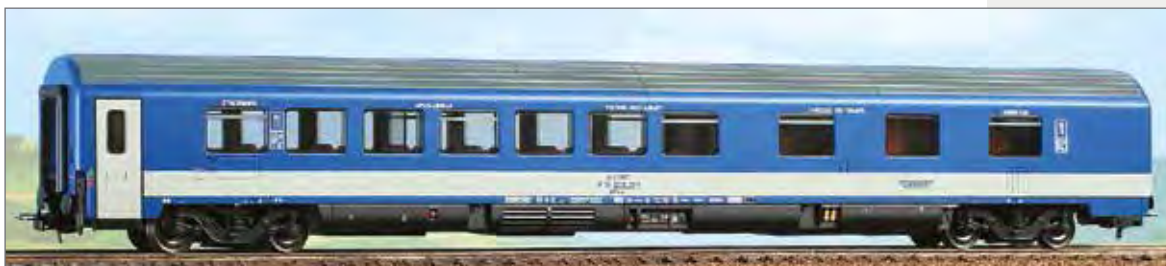
Carrozza ristorante Tipo EuroCity delle MÁV (Ferrovie Statali Ungheresi). Livrea azzurra e bianca. Type EuroCity restaurant car of the MÁV (Hungarian State Railways). Light blue and white livery. Speisewagen Typ Eurocity der MÁV. Blauweiße Lackierung.
